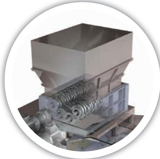
Optional sound-suppressing hopper can provide a significant reduction in operating noise levels.
