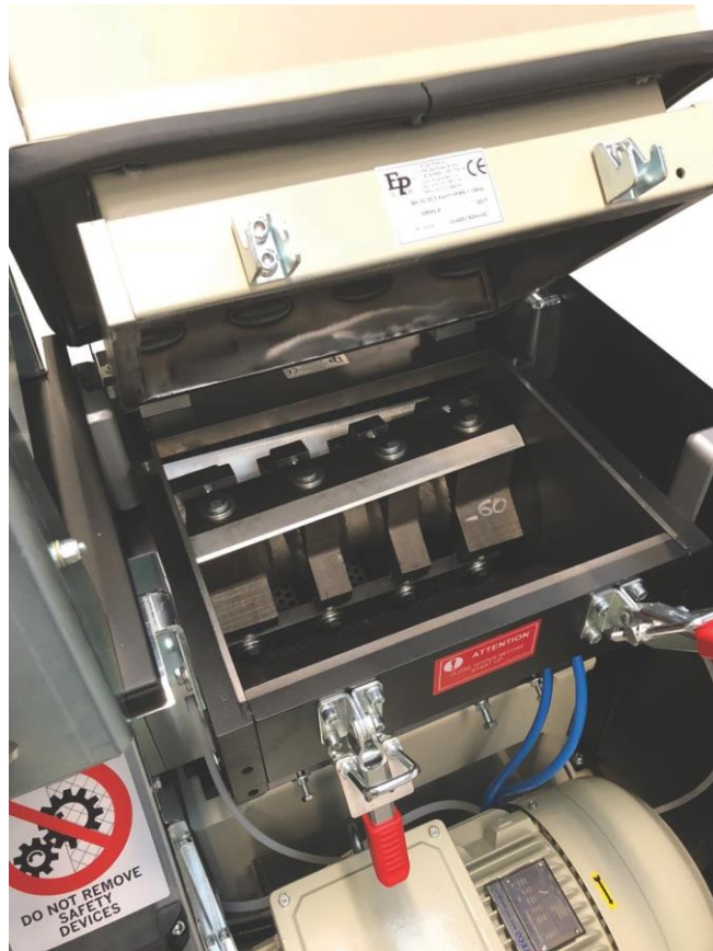
Cutting chamber access point for blade adjustment & blue pipes for water-cooled option
