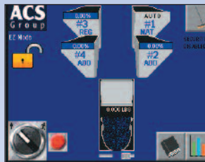
Programmable entry screens for all three recipe modes (up to six components)
