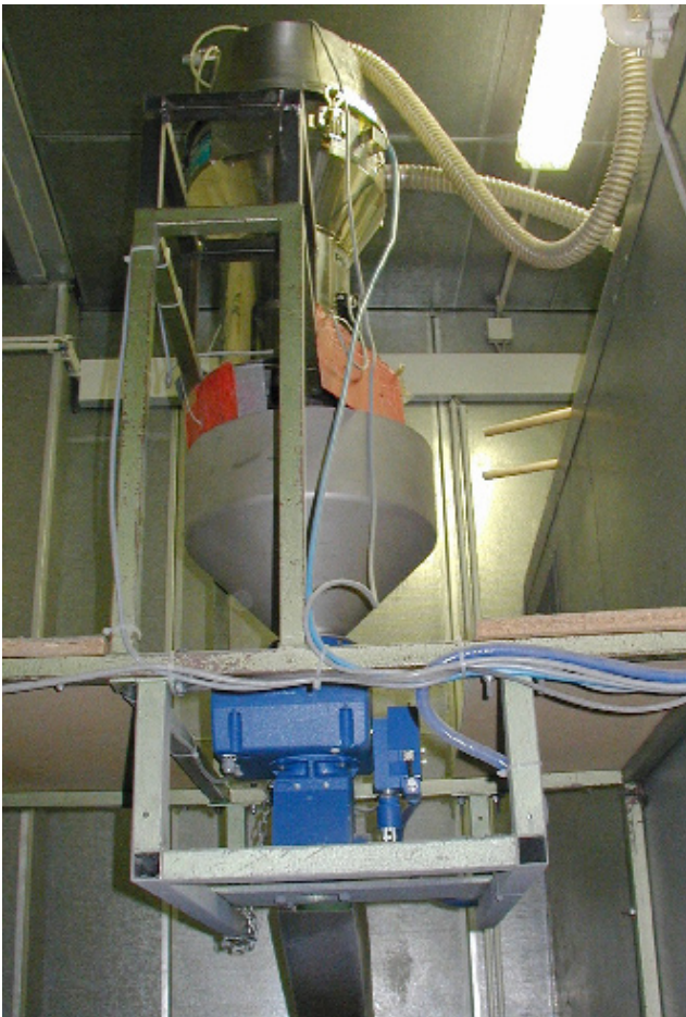
MESEP SE 50 for the inspection of granulates in the plastics industry.
